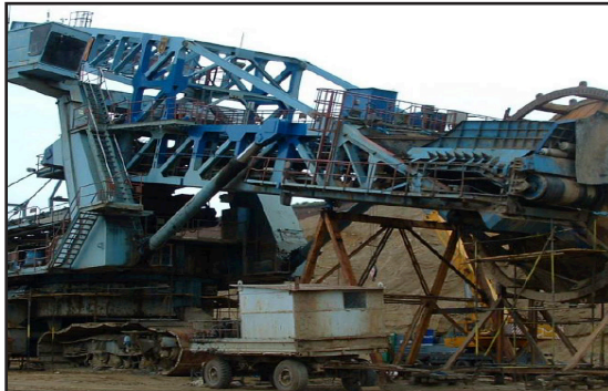
Compact lignite bucket-wheel excavator.
